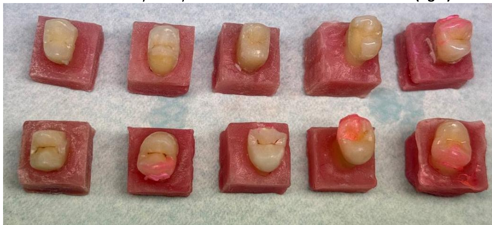
figure (2) sample containing base from self-cure acrylic
